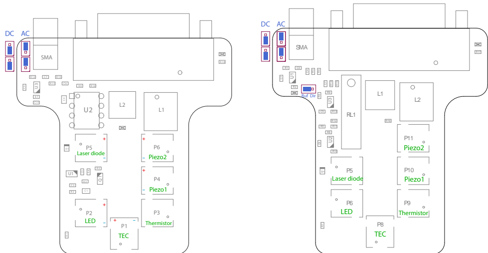
Figure I.4: B1047 (left) and B1240 (right) enhanced laser head boards. Jumpers at top left can be configured for AC or DC coupling. The B1240 has an additional jumper “Buf Dir” for buffered or direct input, shown connected for buffered; change to pins 1 and 2 for direct. Modulation input via SMA connector, sensitivity 2.5 mA/V. Connectors are Hirose DF59.
