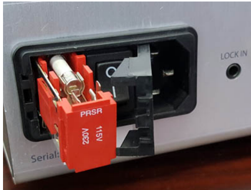
Figure D.1: Fuse cartridge, showing fuse placement for operation at 230 V.
