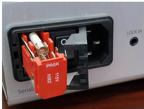
Figure E.1: Fuse cartridge, showing fuse placement for operation at 230 Vac.
