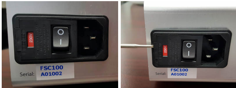
Figure E.2: To change fuse or voltage, open the fuse cartridge cover with a screwdriver inserted into a small slot at the left edge of the cover, just to the left of the red voltage indicator.
