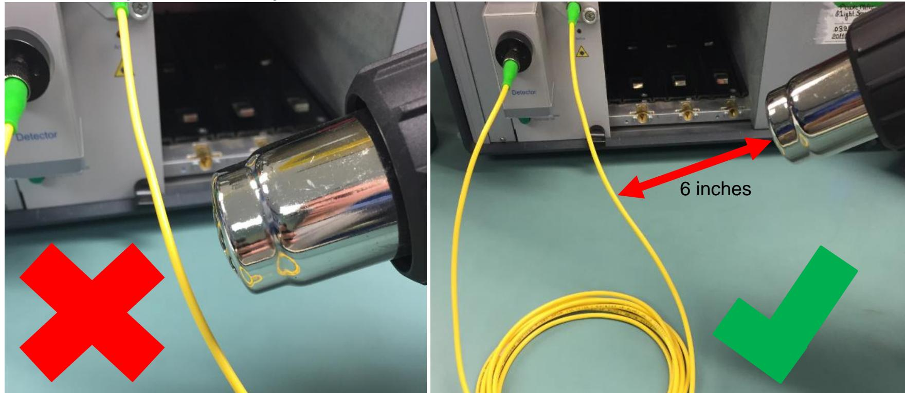
DO NOT hold the heat gun too close to the fiber. It will melt the fiber. Hold the heat gun approximately 6 inches (15cm) away from the fiber.
