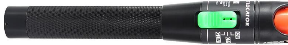
Figure 4.3: Fibre laser pen, or visual fault locator. Injects visible laser beam into fibre, which allows basic alignment and mode matching.
