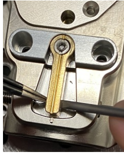
Figure 4.1: Removing the intracavity filter assembly.
