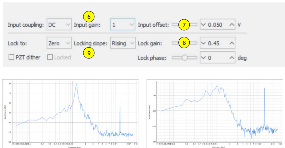
Figure 6.2: mLC locking controls: (6) input gain, (7) input offset, (8) lock gain, (9) locking slope, and error signal spectrum when the control loop gain is too high (lower left) and optimal (lower right).
