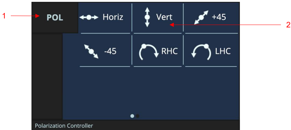
Figure 5: PCU-200 touch screen preset states of polarization
