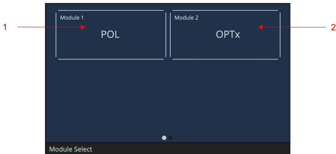
Figure 6: PCU-200 touch screen Module Select page
